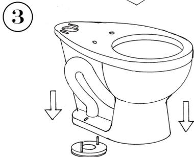
Carefully lower the toilet bowl onto the floor flange while aligning the "T" bolts through the two holes in the toilet bowl foot.
